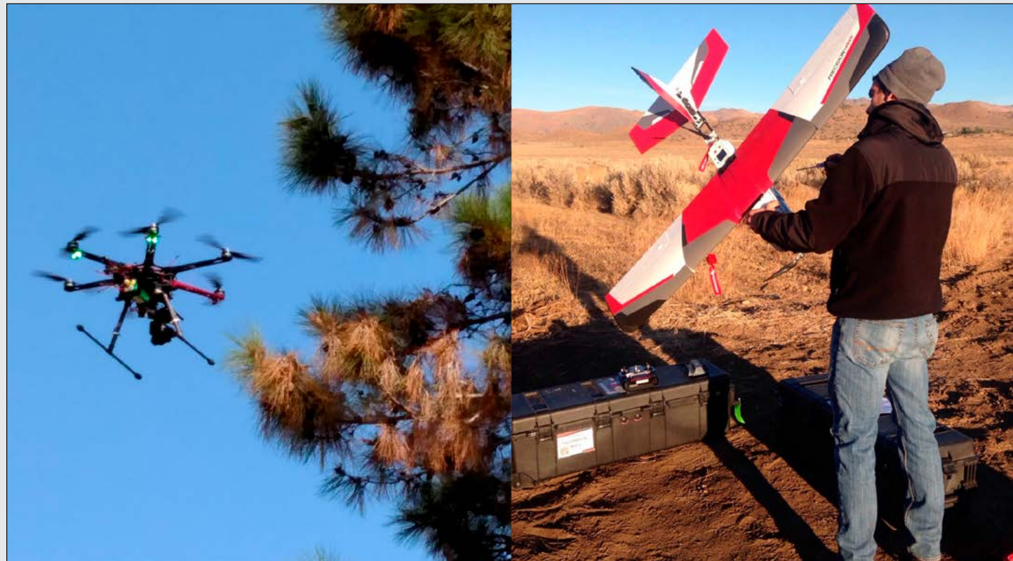
The two main types of UAVs in 2016, rotor-wing (photo courtesy author) and fixed-wing (courtesy PrecisionHawk).
