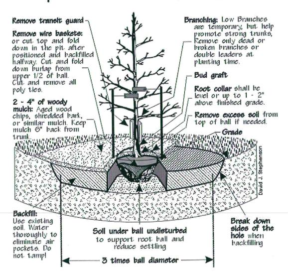
Stake only if you have to. Use 3"-wide webbing straps and secure to stakes with heavy gauge wire. The wire should be able to stick straight out from the stake and hold the webbing strap up, preventing it from sliding down the tree. Do not stake tightly - trees gain strength from movement. Remove all stakes after one year.
