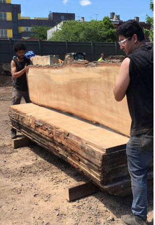
Evaluating, milling, and drying logs at Greenwood Cemetery
