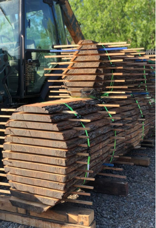
Evaluating, milling, and drying logs at Greenwood Cemetery
